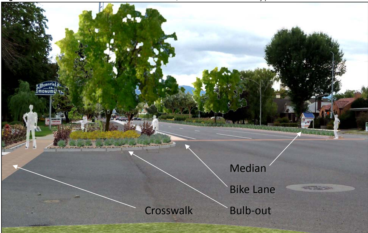
Figure 4-8 AFTER: Illustration of 200 North and Main Street with complete street elements and traffic calming devices
