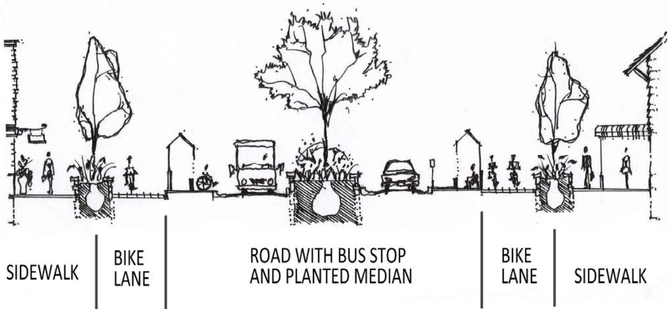
Figure 4-6 section of a Complete Street COMPLETE STREETS: roadways designed and operated to enable safe, attractive, comfortable access to all users
