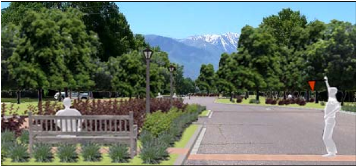
Figure 4-16 AFTER: The same street after plantings were added; vegetated islands were added in such a way as to give the formerly wide road a gentle curve, further calming traffic, this is a traffic calming device known as a chicane
